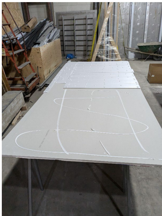
Figure 2 – Gypsum board (1 of 2) and specimen planks with adhesive applied
