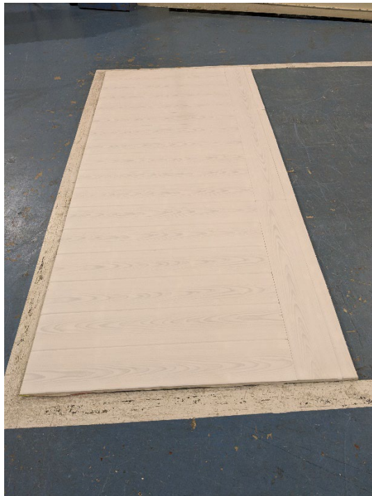
Figure 3 – Gypsum board (1 of 2) with specimen planks installed
