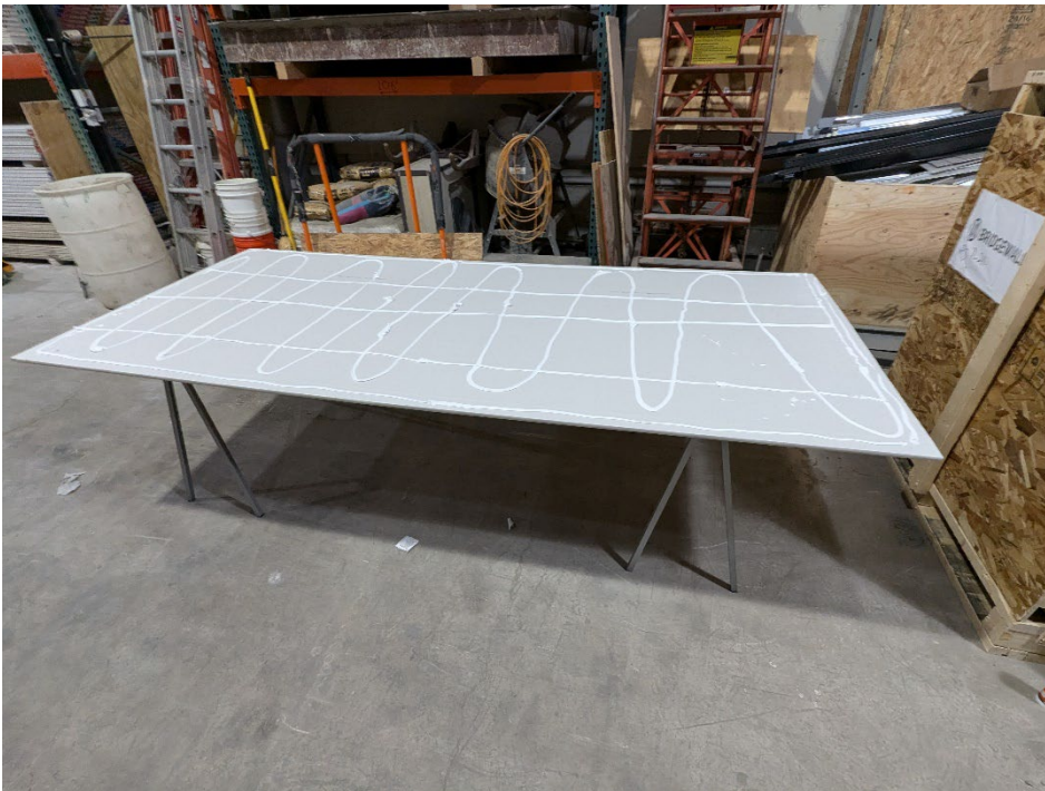
Figure 2 – Individual gypsum board (1 of 2) with adhesive applied to panel
